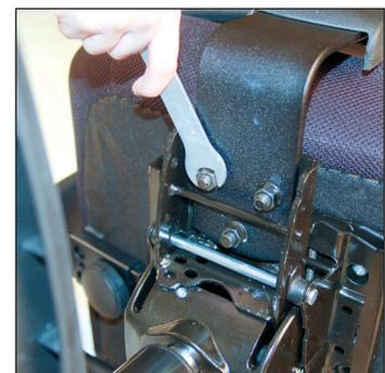
3. With nuts started by hand, tighten all to secure the back assembly to the mechanism.
