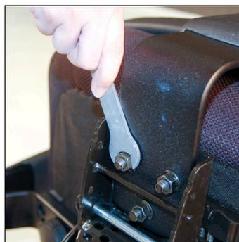
2. Position new backrest and post assembly into the same receptacle/stub. Start the 3 nuts by hand to avoid cross-threading.
