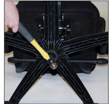
3. Hold the base with one hand and use a plastic or rubber hammer in the other to strike cylinder protruding through the base. The shock force will dislodge the base. If any casters come out of the base, you can easily reinsert them.
