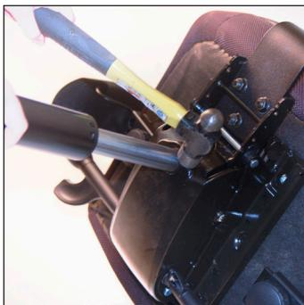
4. Remove cylinder from mechanism: Hold the end of the cylinder with one hand, and hammer the mechanism around the cylinder entry point. Several strong blows may be required to dislodge the cylinder from mechanism.
