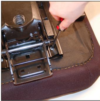
7. With all 4 Phillips screws revealed and removed the mechanism can now be lifted off the seat.
