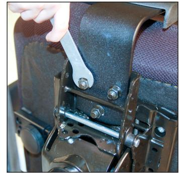
9. Reattach backrest with the 3 bolts and nuts, and then, replace the black, plastic cover.
