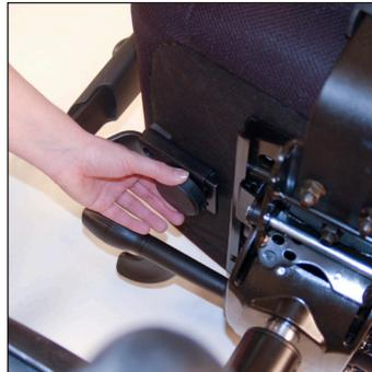
2. Locate where arms attach to underside of the seat, and remove the hand-wheel. Keep all washers in place for later reinstallation.
