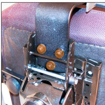
1. To remove backrest, first remove the black, plastic cover where back post meets mechanism. Next, locate and remove the 3 (3/16") nuts that secure backrest post there. Once detached, set aside for later reinstallation.
