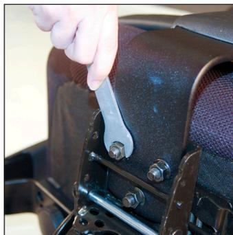
5. To remove backrest, first remove the black, plastic cover where back post meets mechanism. Next, locate and remove the 3 (3/16") nuts that secure backrest post there. Slip the bolts up and out and set aside for later reinstallation.
