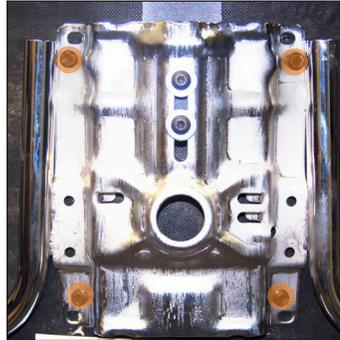
1. To remove the seat, access the underside of the chair, locate and remove the 4 (3/8") Hex-head bolts that secure the seat to the mechanism.
