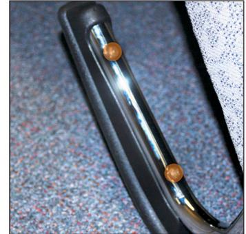
1. To remove urethane arm pads, access the underside of the arms, locate and remove the 2 Phillips-head screws secure the pads to the frame.
